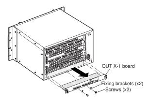
4. Mount the network board into the OUT X-1 slot, and fix the board with the supplied screws.
